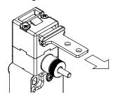
The inside of each switch features a device which holds the actuator in its closed position. Ideal for all those applications where several doors are unlocked simultaneously, but only one is actually opened. The device keeps all the unlocked doors in their position with a retaining force of 30 N $\sim$ , stopping any vibrations or gusts of wind from opening them
