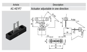
Actuator adjustable in one direction for doors with reduced dimensions.
