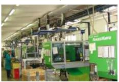
POLYCOM is a rapidly growing supplier of advanced plastic parts and molding tools. It employs the CyBro subsystem to ensure automatic output count, on-line monitoring of machine cycle time, consistent monitoring of on-spot standstills / halts, and real-time data processing.
