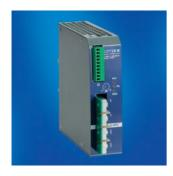
Battery test/monitoring is cyclic I-U<sub>0</sub>-U charge with car charge level temperature compensated charging voltage deep discharge protection (residual discharge current <300 uA) electronic battery short-circuit protection control by state-of-the-art digital technology signalling via LEDs, relays fault diagnosis (battery temperature, aging, cable break, etc.) Option: fast charge by means of power supply bypass
