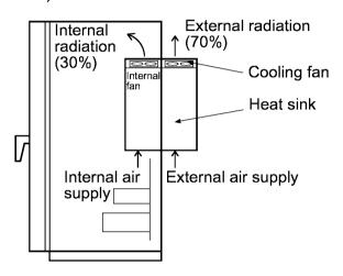
Figure 2-2-2 External cooling system
