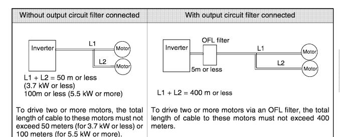
Note: When a motor protective thermal O/L relay is inserted between the inverter and the motor, the thermal O/L relay may malfunction (particularly in the 400 V series) even when the cable length is 50 meters or less. To resolve, insert an OFL filter or reduce the carrier frequency of the inverter operation noise. (Use function code "F26 Motor sound".)
