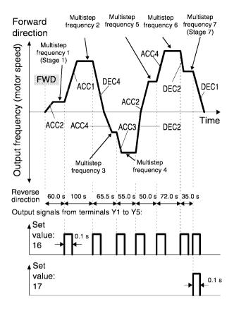
Running and stopping are controlled by pressing the FWD and STOP keys and by opening and closing the control terminals.
