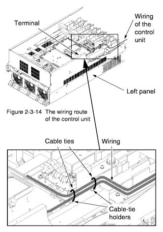
Figure 2-3-15 The securing points of the cables
