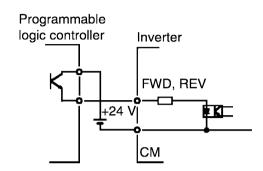
Figure 2-3-11 Connection for External power supply
