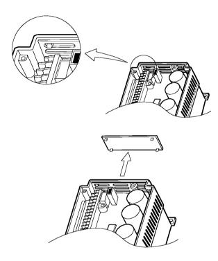
Figure 2-2-4 Removing the ventilating cover
