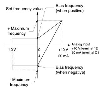
When this function is used with function F17 (bias frequency), the gain set with this function is valid and the gained frequency is biased.
