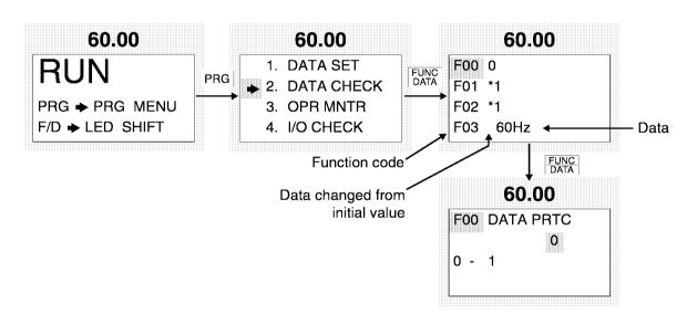
Select the desired function and press  $\frac{\text{FUNC}}{\text{DATA}}$  to check the function data. By pressing  $\frac{\text{FUNC}}{\text{DATA}}$ , the screen switches to the "DATA SET" screen, to modify data.
