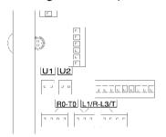
When shipped from the factory, CN UX is connected to the  $\boxed{\text{U1}}$  side and CN RXTX is connected to the  $\boxed{\text{L1/R-L3/T}}$  side.
