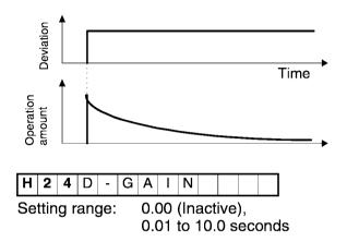
"H24 D-gain" is used as a parameter to determine the effect of a D operation. A longer differentiation time causes vibration by P operation quickly attenuating at the occurrence of deviation. Excessive differentiation time could cause vibration. Shortening the differentiation time reduces attenuation at the occurrence of deviation.
