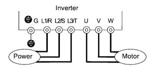
Figure 3-1-1 Inverter connection
