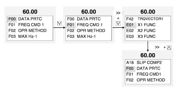
Select the desired function and press FUNC to switch to the "data setting" screen.
