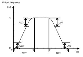
100% value of this function means maximum frequency (fmax).
