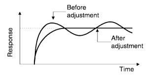
To suppress vibration with a frequency roughly equivalent to the value "H24 D-gain," decrease the value of H24. If there is residual vibration with 0.0, decrease the value of "H22 P-gain."
