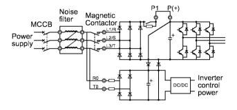
Figure 2-3-2 Connecting the auxiliary control-power input terminals
