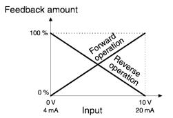
Only positive values can be input for this feedback amount of PID control.
