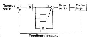
Forward or reverse operations can be selected for PID controller output. This enables motor revolutions to be faster or lower according to PID controller output.
