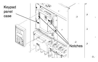
Figure 1-3-4 Removing the keypad panel (for inverter of 30 kW or more)
