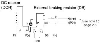
Figure 2-3-4 Connection (7.5 kW or less)
