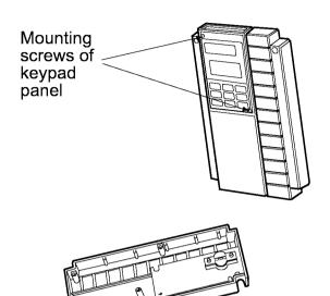
Figure 1-3-3 Removing the keypad panel
