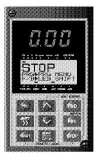
Figure 3-1-2 Display on keypad panel at power-on
