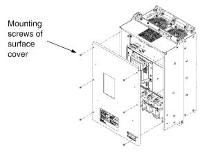
Figure 1-3-2 Removing the surface cover (for inverter of 30 kW or more)
