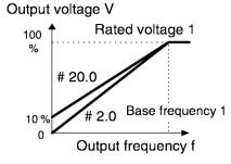
**Note:** As a large torque boost value creates overexcitation in the low-speed range, continued operation may cause the motor to overheating. Check the characteristics of the driven motor.
