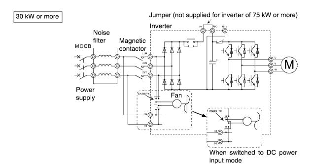
Figure 2-3-6 Fan power switching
