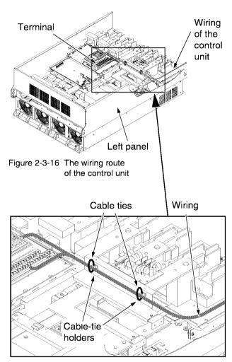
Figure 2-3-17 The securing points of the cables
