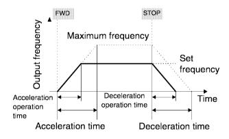
Note: If the set acceleration and deceleration times are too short even though the resistance torque and moment of inertia of the load are great, the torque limiting function or stall prevention function becomes activated, thereby prolonging the operation time beyond that stated above.
