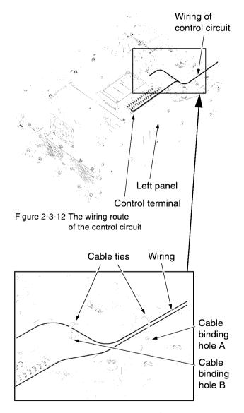
Figure 2-3-13 The securing positions of the control-circuit line of inverter
