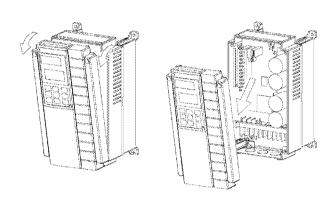
Figure 1-3-1 Removing the surface cover (for inverter of 22 kW or less)
