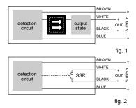
The DECOUT® output is also able to switch the output state at rest from NO to NC and vice versa simply by reversing the polarity of the power supply cables (BROWN - BLUE). Therefore, it is possible to perform all the output configurations, as shown in fig. 3.
