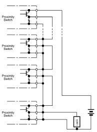
Series Connection of DC Switching Type Proximity Switches (PNP)
