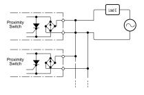
Parallel Connection of AC Switching Type Proximity Switches
