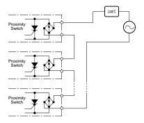
Series Connection of AC Switching Type Proximity Switches
