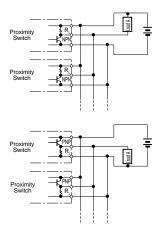
Care must be taken that the combined leakage currents of all proximity switches in parallel is not sufficient to maintain the load in the 'on' state.
