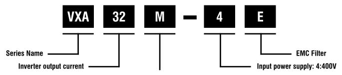
Protection structure: M:IP21 L:IP55 S:IP00
