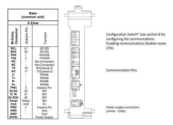
${\sf SS: Chip \, Select \, pins. \, These \, pins \, can \, act \, as \, {\sf TTL}, \, so \, they \, can \, work \, for \, the \, {\sf Chip \, Select \, pin \, of \, any \, device.} }$
