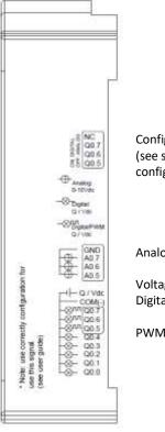
Configuration Switch\* (see section 8 to select the correct configuration for outputs).
