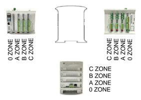
• The inputs in the zone A/B/C are named IX.X, being X any number suitable in the Shield. Outputs are named as QX.X.
