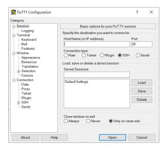
For setting up PuTTY the Raspberry IP must be entered on the *HostName* field and make sure that the port 22 is being used and the *SSH* option is selected on the *Connection Type*. After all the settings have been done, click on the *Open* button to run the program. For a faster start in subsequent sessions, before run the program, enter a name on *Saved Sessions* and click on the *Save* button (a double click on the named configuration will execute the program with the saved configurations).
