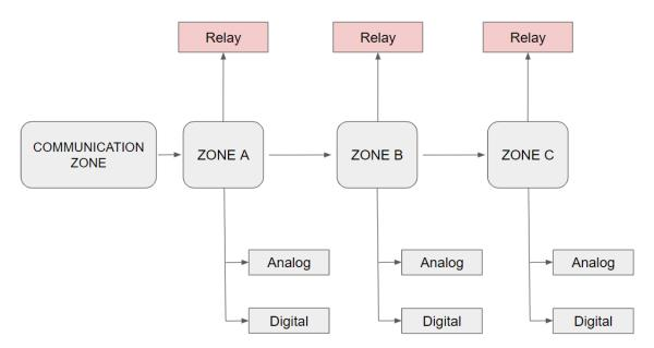
This is the possible zones scheme, whether the zone is Analog/Digital or Relay depends on your device, you can consult it on the <u>Zones Table</u>. The distribution of the different features that provide the Raspberry PLC Family are described below.
